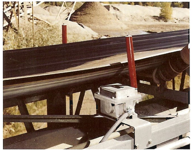
Always used in pairs, the TA conveyor belt alignment switch protects conveyor belts from damage due to belt misalignment or runoff.
